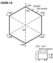
Quantity Tested: 5 units Test Method: Shock was applied 3 times in 6 directions along 3 axes and the level at which shock caused malfunction was measured. Rating: 100 m/s<sup>2</sup>
